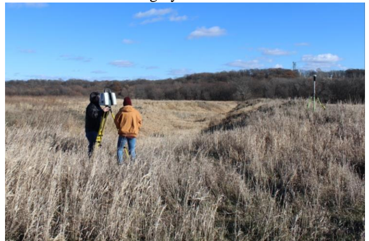
Figure 1: University of Iowa students Drew Hutchinson (left) and Natalie Schoen (right) scan a large drainage ditch using the terrestrial lidar unit. A ground control point to the right establishes standard measurements for the device as it scans.
